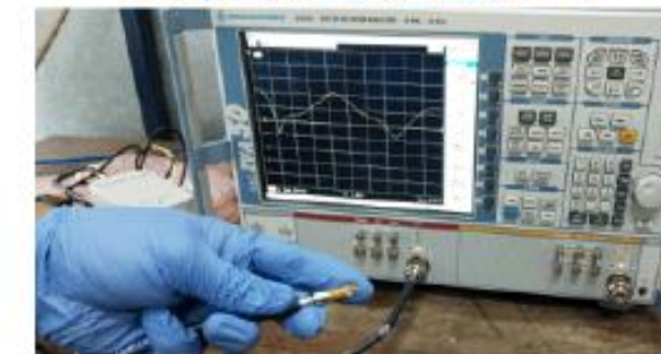
S_{11} Measurement Set-up on Finger, Wrist, Chest, and Thigh using VNA
