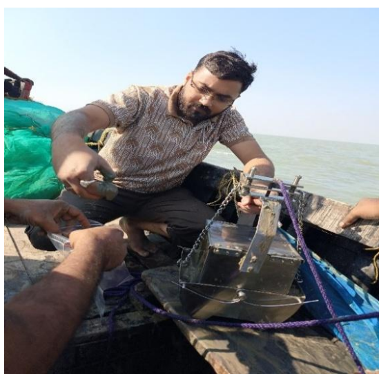
Prof. A. K. Bhaumik and his group collected grab samples using Van-Veen Grab sampler and measured ocean water physical parameters using CTD meter at Digha offshore, Bay of Bengal.
